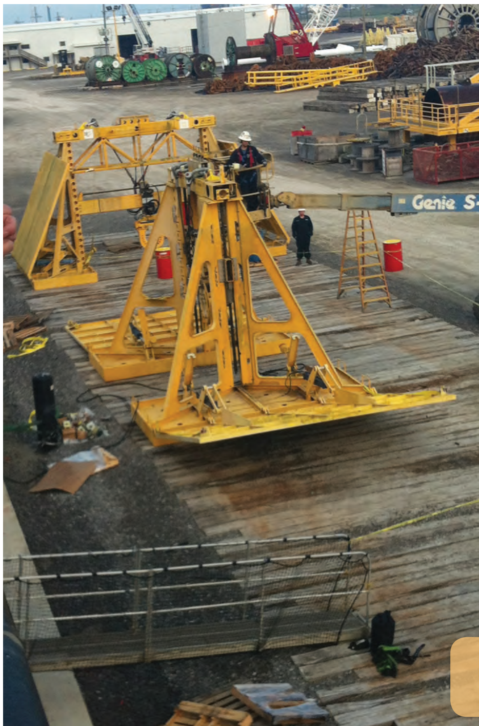
A pipe lifting frame at the quayside undergoing functional testing before deployment.
